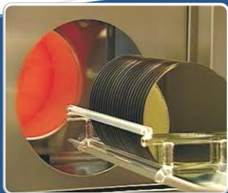
2" through 300mm Diameter Wafers Dry and Wet Thermal Oxidation 500Å Through 5µm Thicknesses Standard \pm 5\% Uniformity
